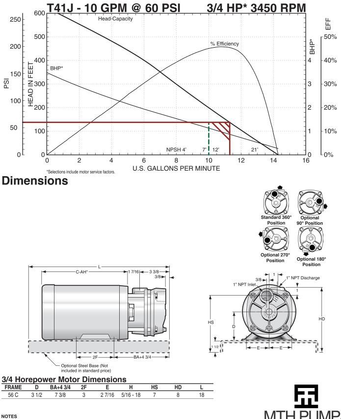
All dimensions in inches. May vary ± 1/4 inches. Not for construction purposes unless certified. \*See motor dimensions for "C-AH" dimension (Varies depending on motor enclosure).
